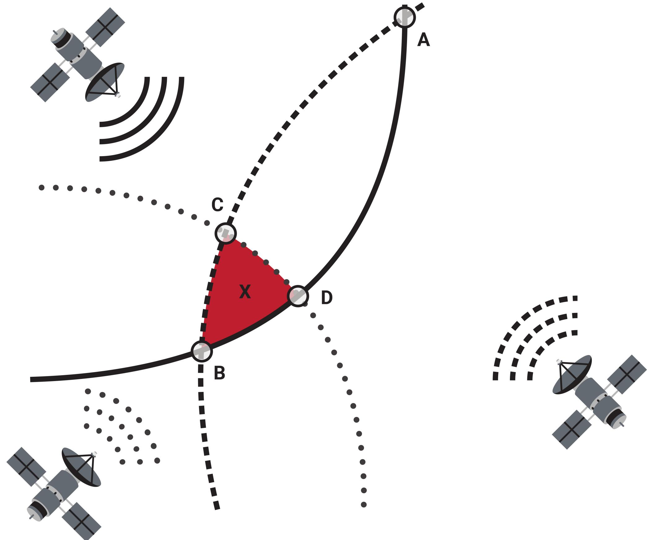
The receiver determines its position (longitude, latitude, altitude) using the principle of trilateration.
