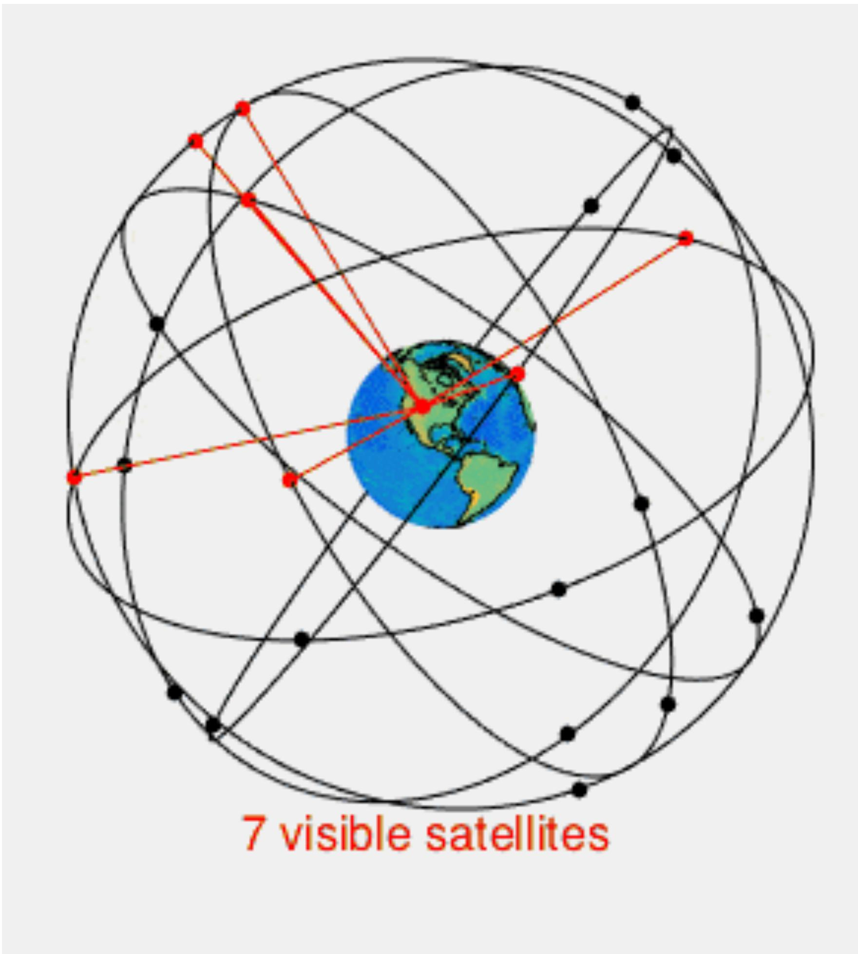
The satellites broadcast a signal with their position and time of transmission.
