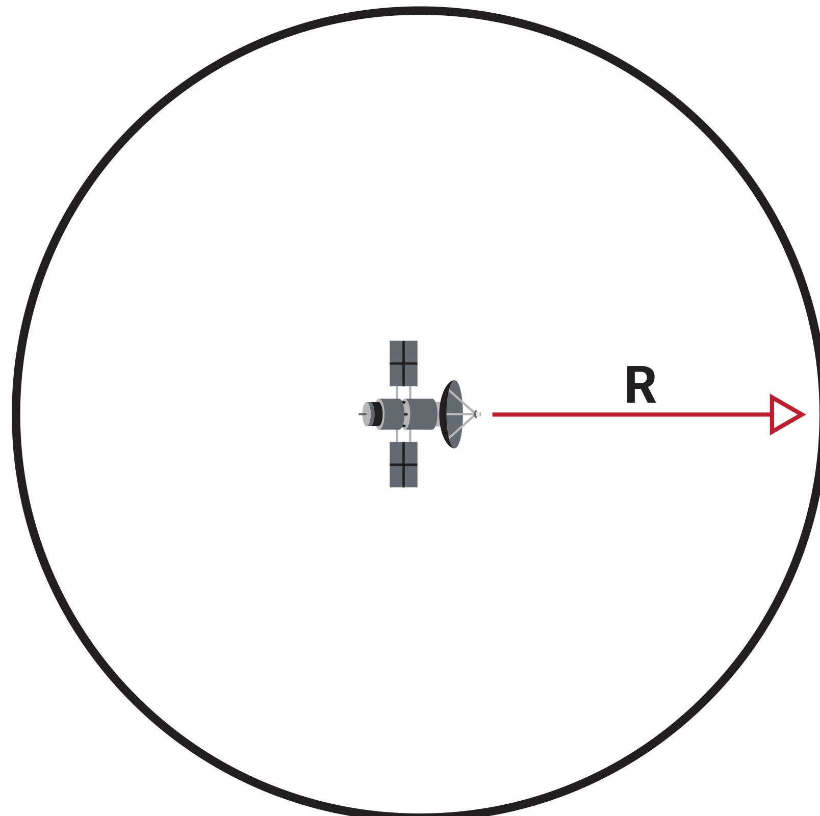
The receiver determines its position (longitude, latitude, altitude) using the principle of trilateration.
